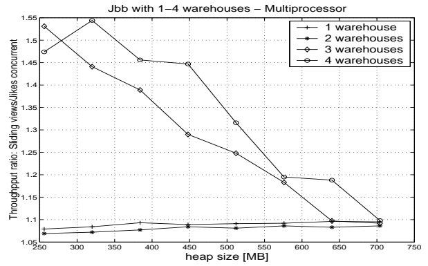
Figure 11: SPECjbb2000 on a multiprocessor: throughput ratio for 1-4 warehouses compared to the Jikes concurrent collector.
